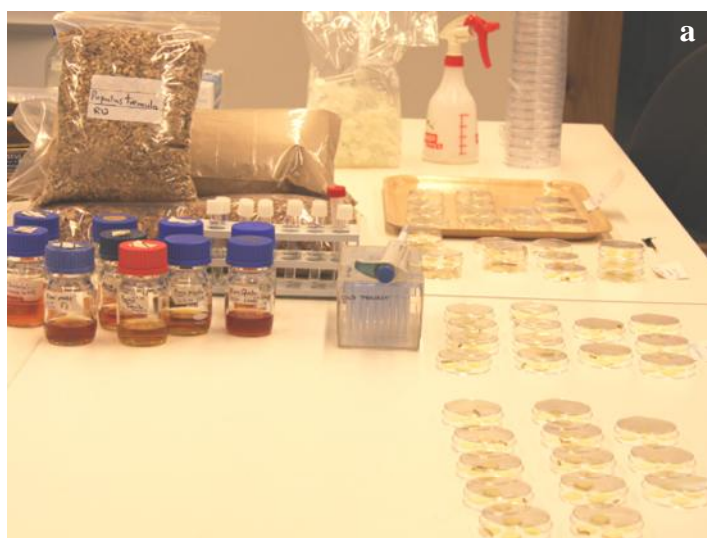
(a) The bark extracts based on water (30/60°C) and absolute ethanol (30°C) solvents, and a choice bioassay in progress in the ForestSpeCs lab at the Department of Agricultural Sciences, University of Helsinki, Finland
